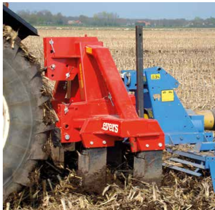
Pre-subsoilers with 4 or 6 tines have a universal PTO channel for mounting a PTO driven machine
