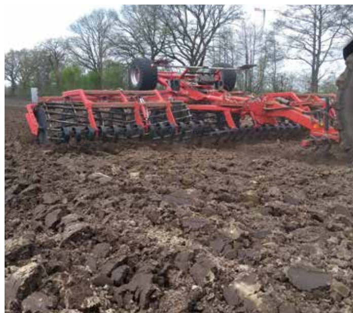
The Concord roller also leaves a level and finely crumbled seedbed, even on heavy soils.
